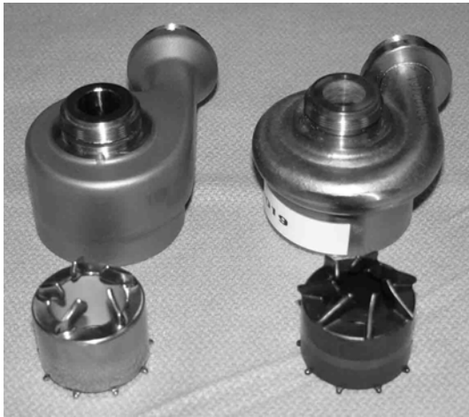
Figure 5. Comparison of DexAide RVAD (left) and CorAide LVAD (right) primary impellers.
